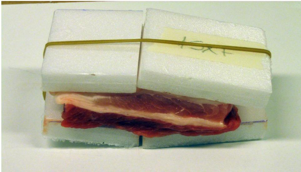
**Fig. (1).** Meat sample with plastic foam slabs. This photo originates from the pre-test series when not totally fat free meat samples were used. The temperature rise of the meat samples with applied insulation, taken from 7°C into room temperature was shown to be approximately 1°C/4 minutes in a pre-experimental test.
