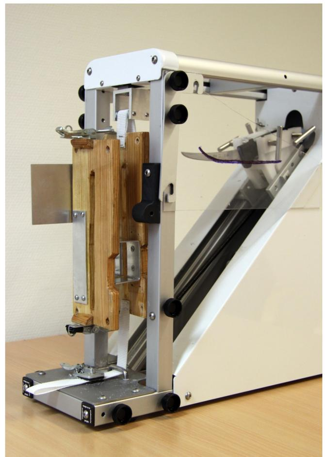
**Fig. (2).** The sharpness testing system pictured with the wooden fixture designed for the study. No meat is inserted in this photo but the knife is shown at the bottom/end position penetrating the 10 mm wide slot.
