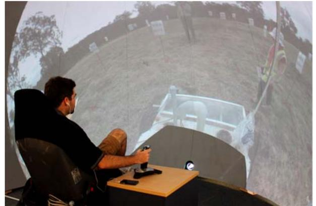
**Fig. (3).** An off-site operator using the dome display.
