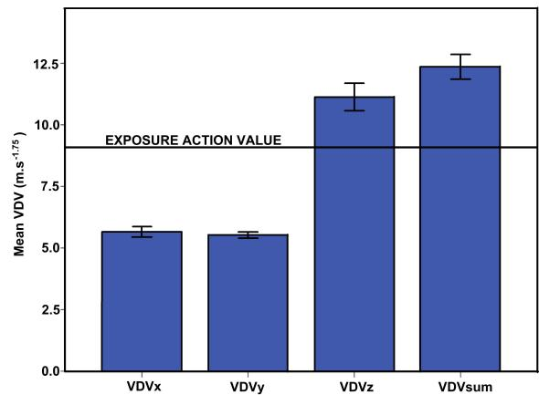
**Fig. (2).** Mean VDV<sub>X</sub>, Y, Z and sum ( $\text{m}/\text{s}^{1.75}$ ) (error bars represent 95% confidence intervals).
