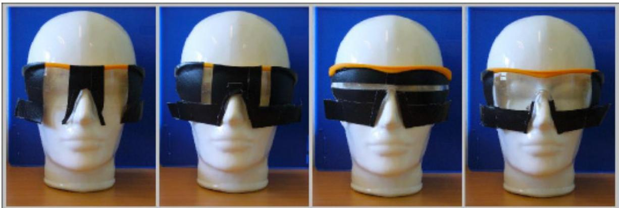
Fig. (1). Four examples of FoV limiting goggles.
