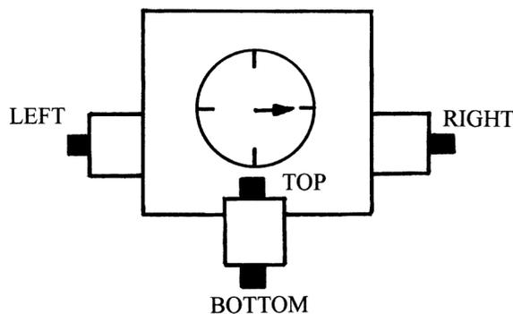
**Fig. (6).** Locations of the controls relative to the display in the experiments of [11,12]. Subjects sat in front of the CRT on which the circular display was presented. Top and right rotary controls are from [11]; Left and Bottom rotary controls are from [12]. Drawing is not to scale.
