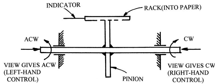
**Fig. (5).** A possible form of 'implied linkage' for the three-dimensional display/control arrangement shown in Fig. (4), when the rotary control is either on the left or right-hand side of the display (Front view).
