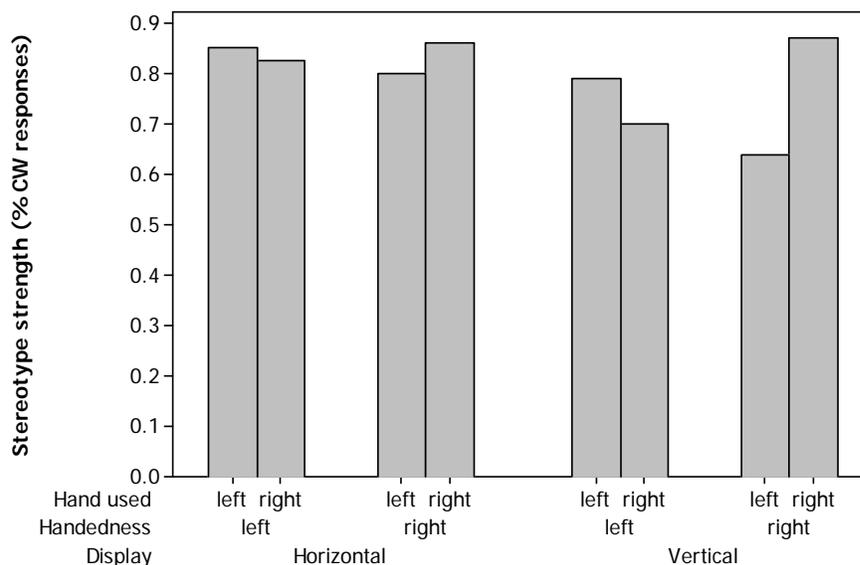
**Fig. (3).** Data of Chapanis and Gropper [10, figure 7, page 315] for left and right-handed subjects using their preferred and non-preferred hands. The display was either orientated horizontally or vertically; the control knob was always in the bottom position.
