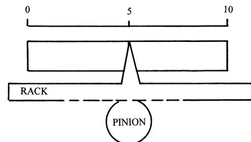
**Fig. (1).** The 'implied linkage' for two-dimensional display/control relationship where Warrick's principle is operational (linear display with rotary control).
