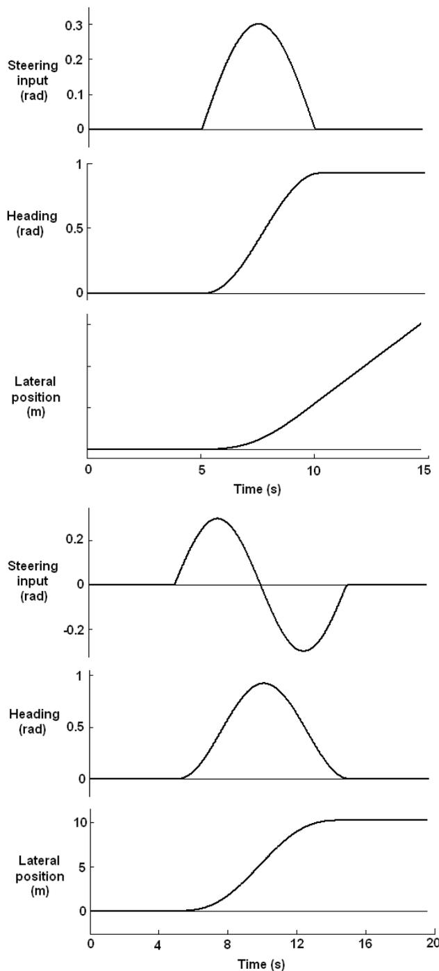
Fig. (5). Steering wheel inputs necessary to perform a simple turn (top) and a lane change (bottom).
