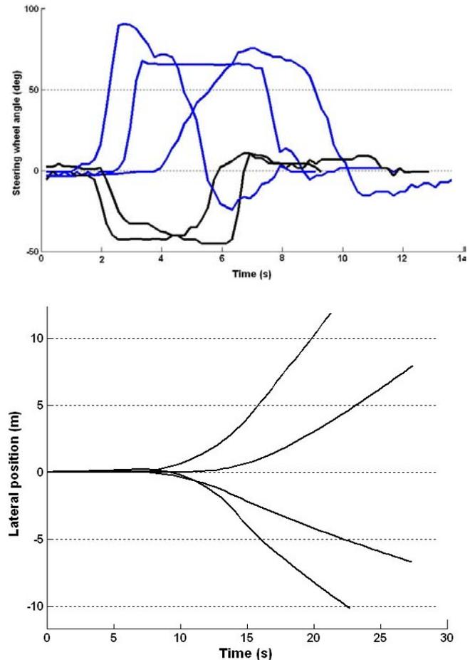
Fig. (6). Steering wheel angle and lateral deviation of the tractor in experiment SE2 as the drivers performed the maneuver 4 in Fig. (1).
