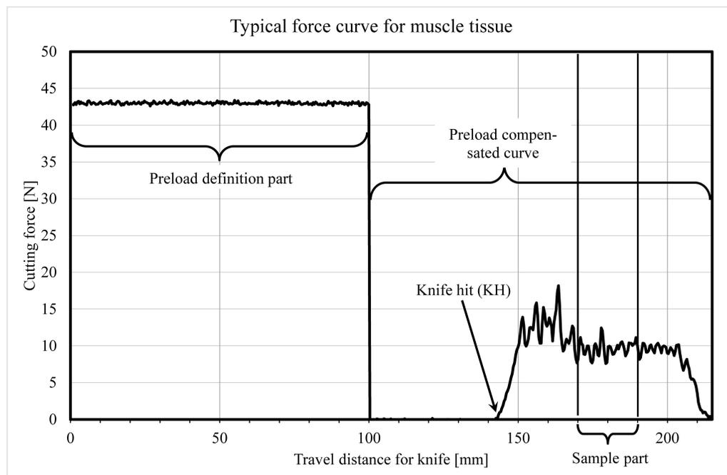
**Fig. (3).** An example of a force curve recorded by the ANAGO sharpness analyzer. The point where the knife stabs the meat sample is indicated (KH) and also the standardized part of the curve used for deducting a sample force average.
