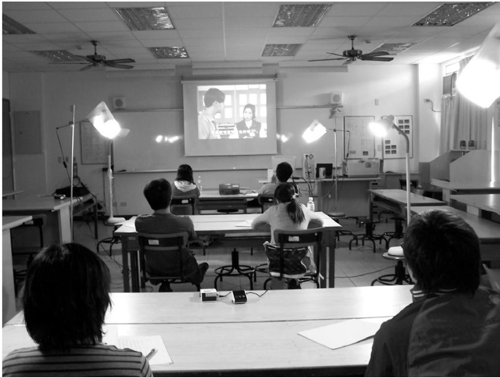
**Fig. (1).** The workplace arrangement used in the experiment. This picture was taken using the 750 lux ambient illumination condition.
