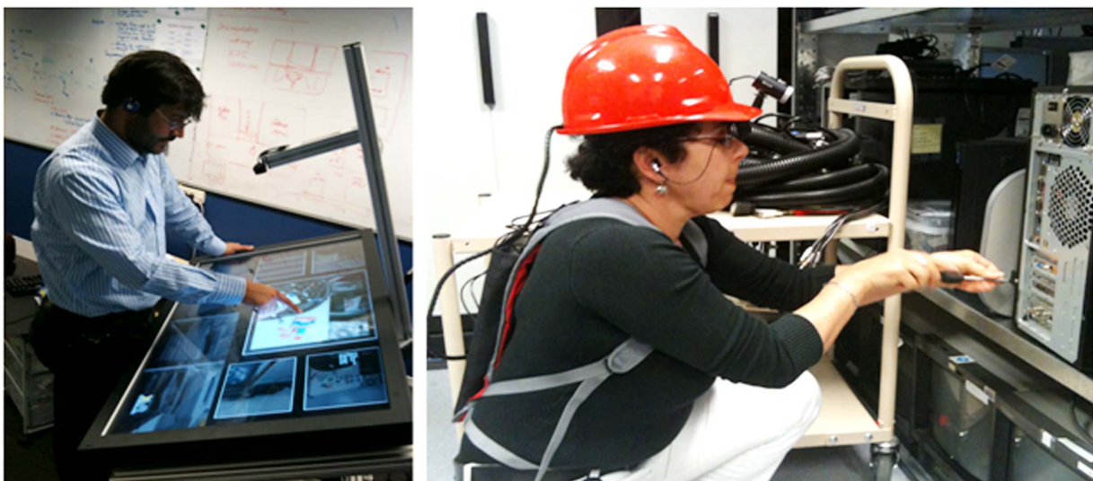
Fig. (8). The helper control console (left) and the worker wearable unit (right).
