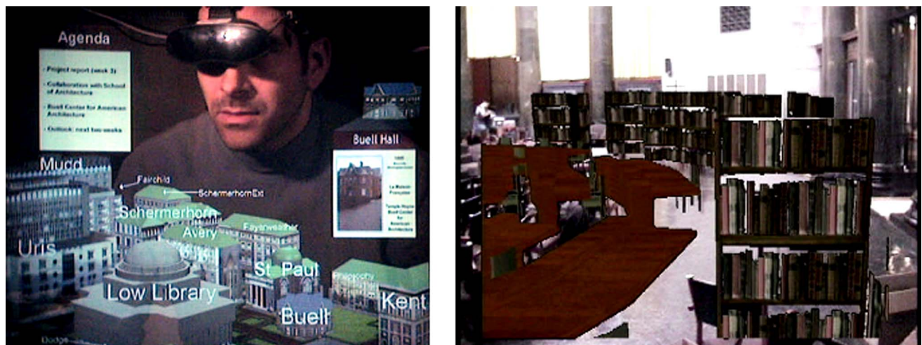
Fig. (6). Optical see-through (left) and Video see through indoor AR (right) [18].
