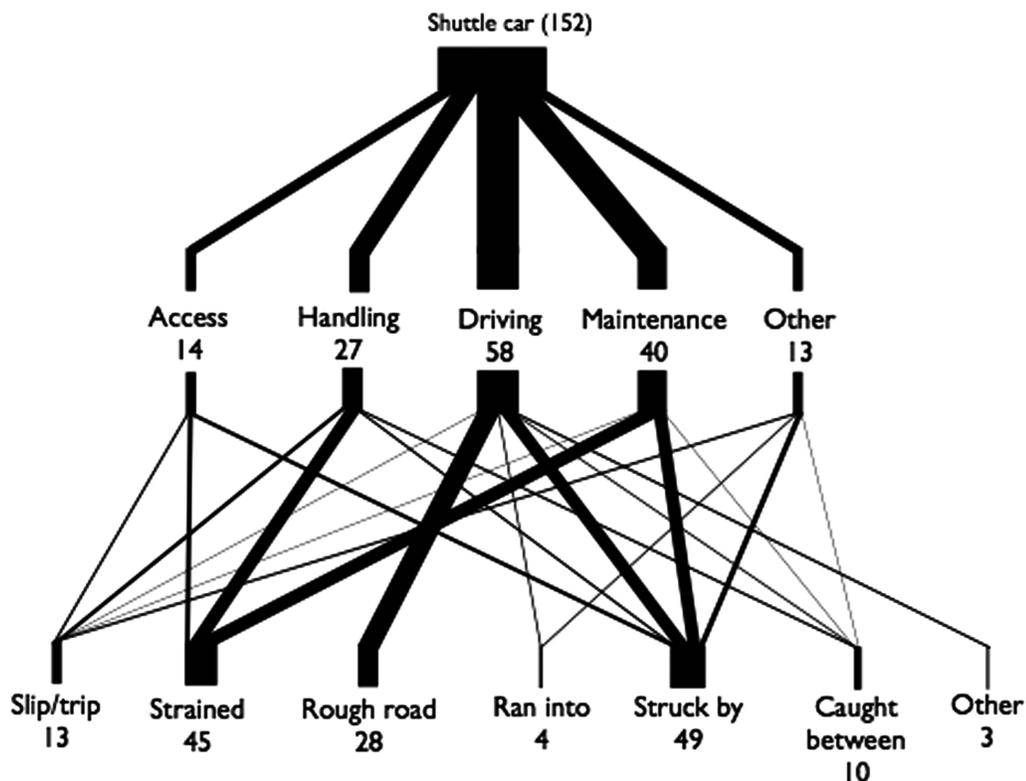
**Fig. (5).** Underground injury frequency by Activity and Mechanism associated with Shuttle cars for NSW mines during the 3 years to June 30, 2008.
