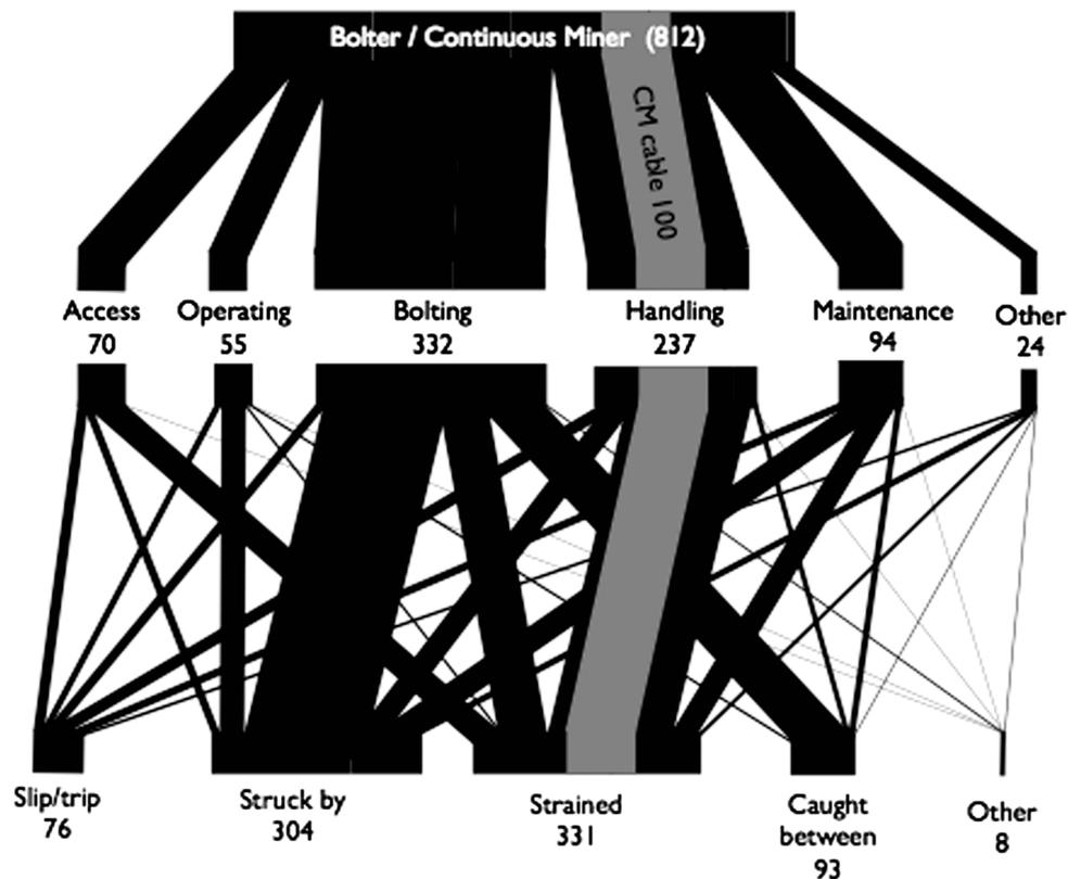
**Fig. (1).** Underground injury frequency by Activity and Mechanism for Continuous Miner and Bolting Machine for NSW mines during the 3 years to June 30, 2008.
