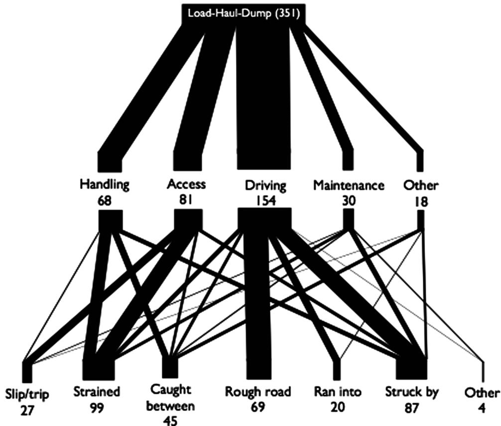
Fig. (2). Underground injury frequency by Activity and Mechanism associated with LHD for NSW mines during the 3 years to June 30, 2008.
