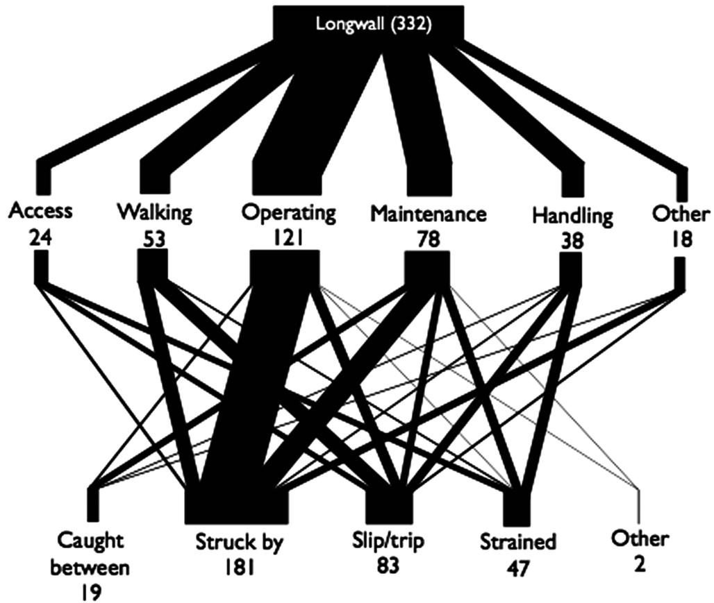
Fig. (3). Underground injury frequency by Activity and Mechanism associated with Longwall equipment for NSW mines during the 3 years to June 30, 2008.
