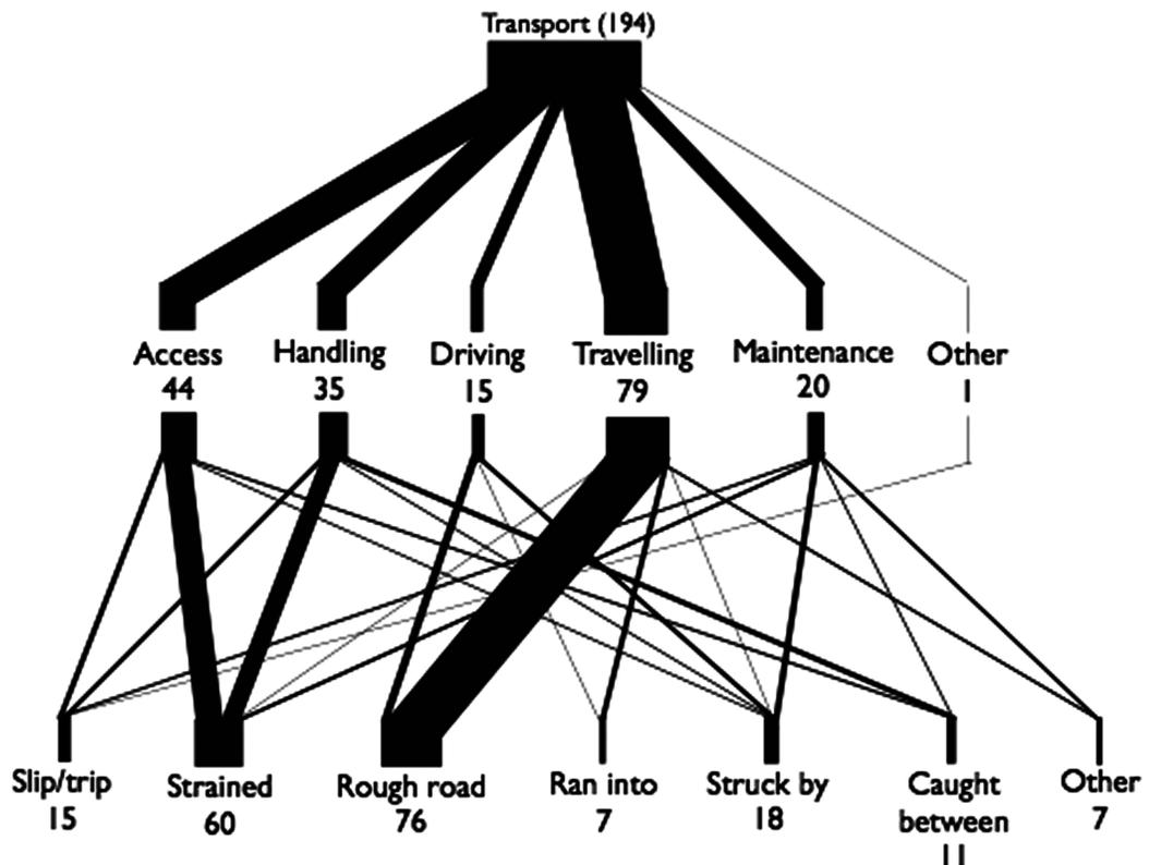
Fig. (4). Underground injury frequency by Activity and Mechanism associated with Personnel transport for NSW mines during the 3 years to June 30, 2008.
