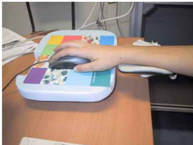
Fig. (1). The measurement of compression forces of the hand on the mice during the mice movements protocol.
