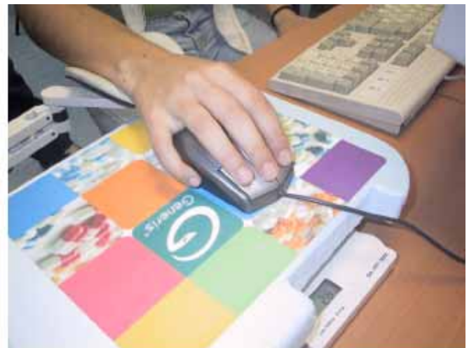
Fig. (1). The measurement of compression forces of the hand on the mice during the mice movements protocol.
