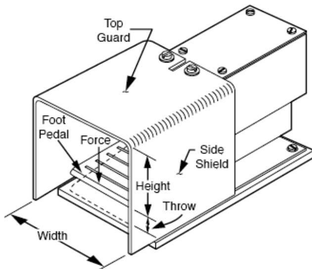
Fig. (2). Foot control characteristics.
